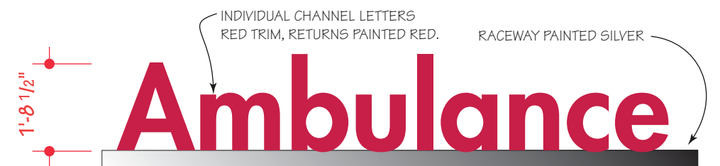
4 FRONT ELEVATION @ AMBULANCE CANOPY - LOCATION 4 3/8" = 1'-0"
