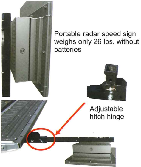
Convenient folding hitch kit with adjustable hinge
