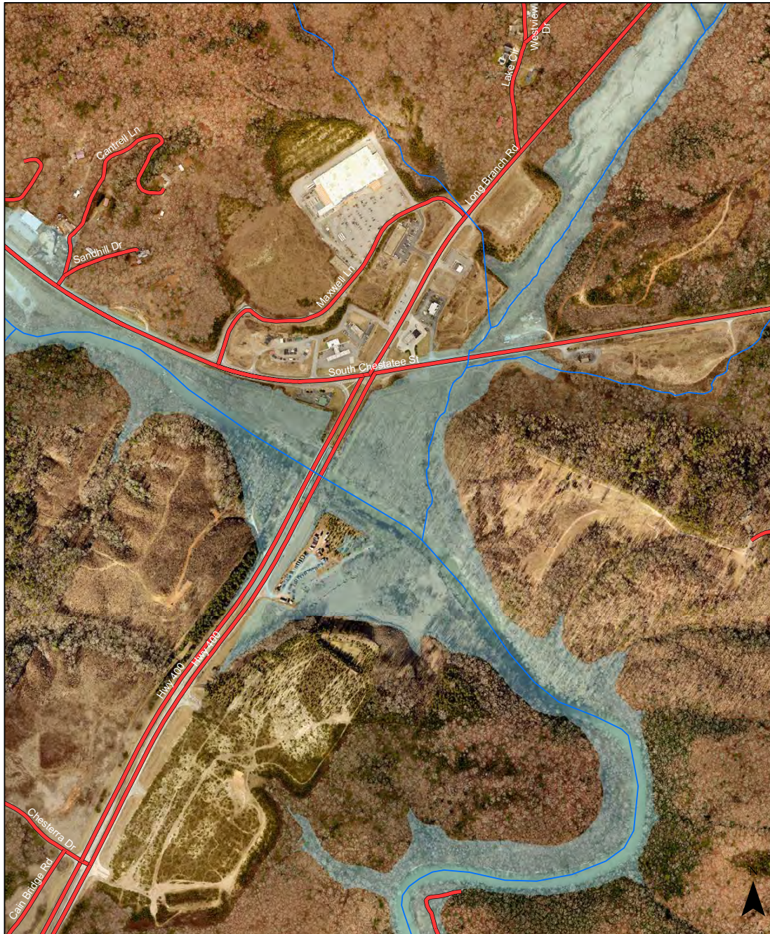
Flooding Concerns 8" over Hwy 60 and Hwy 400
