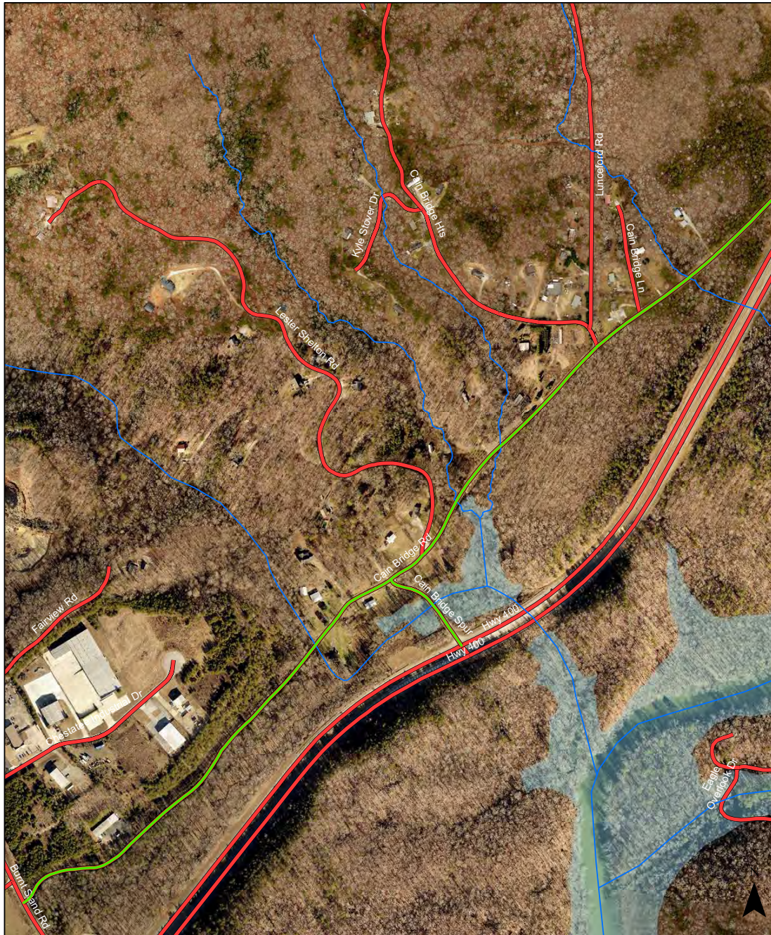
Flooding Concerns 12" over Cain Bridge Rd.
