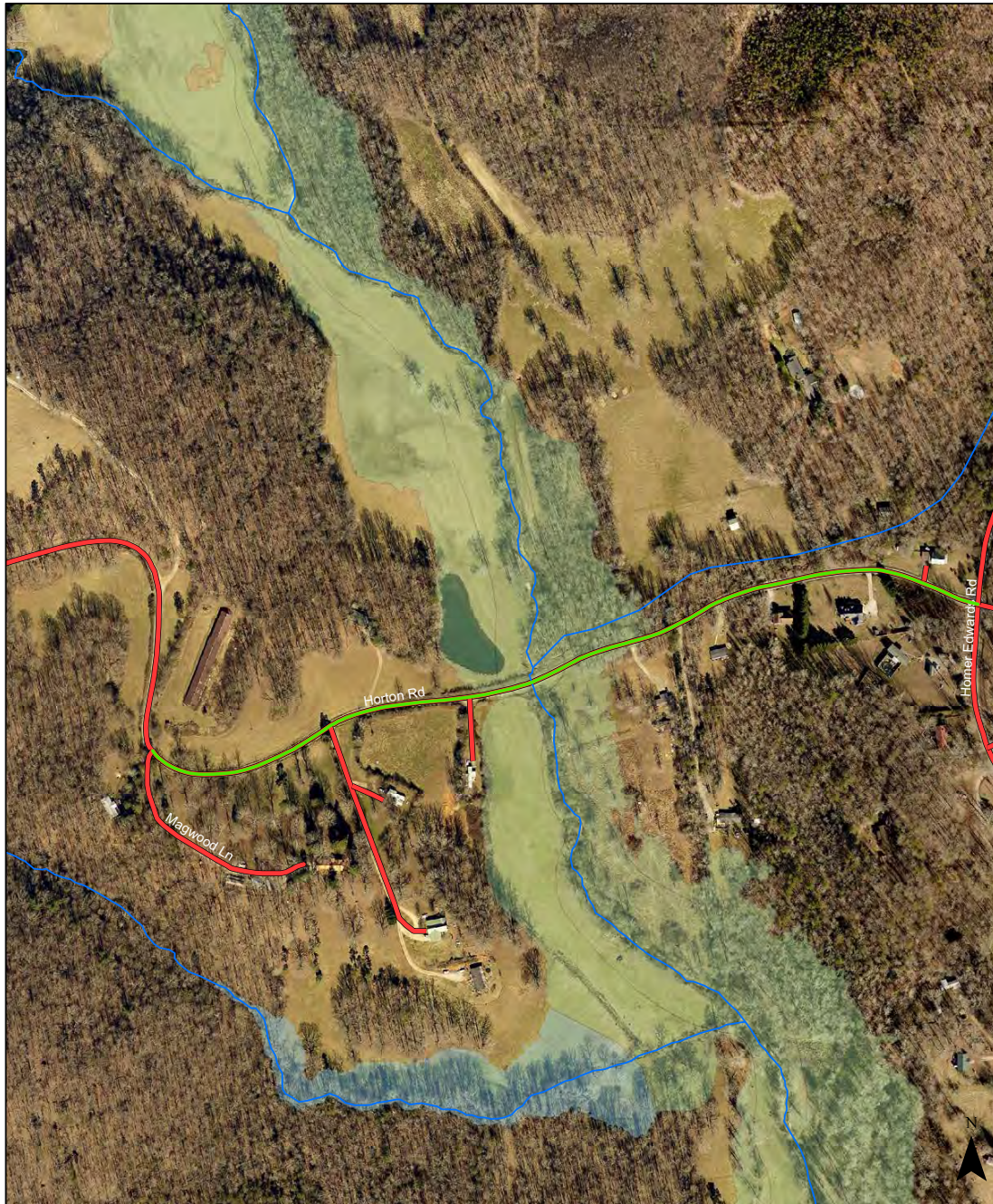
Flooding Concerns 18" over Horton Rd.
