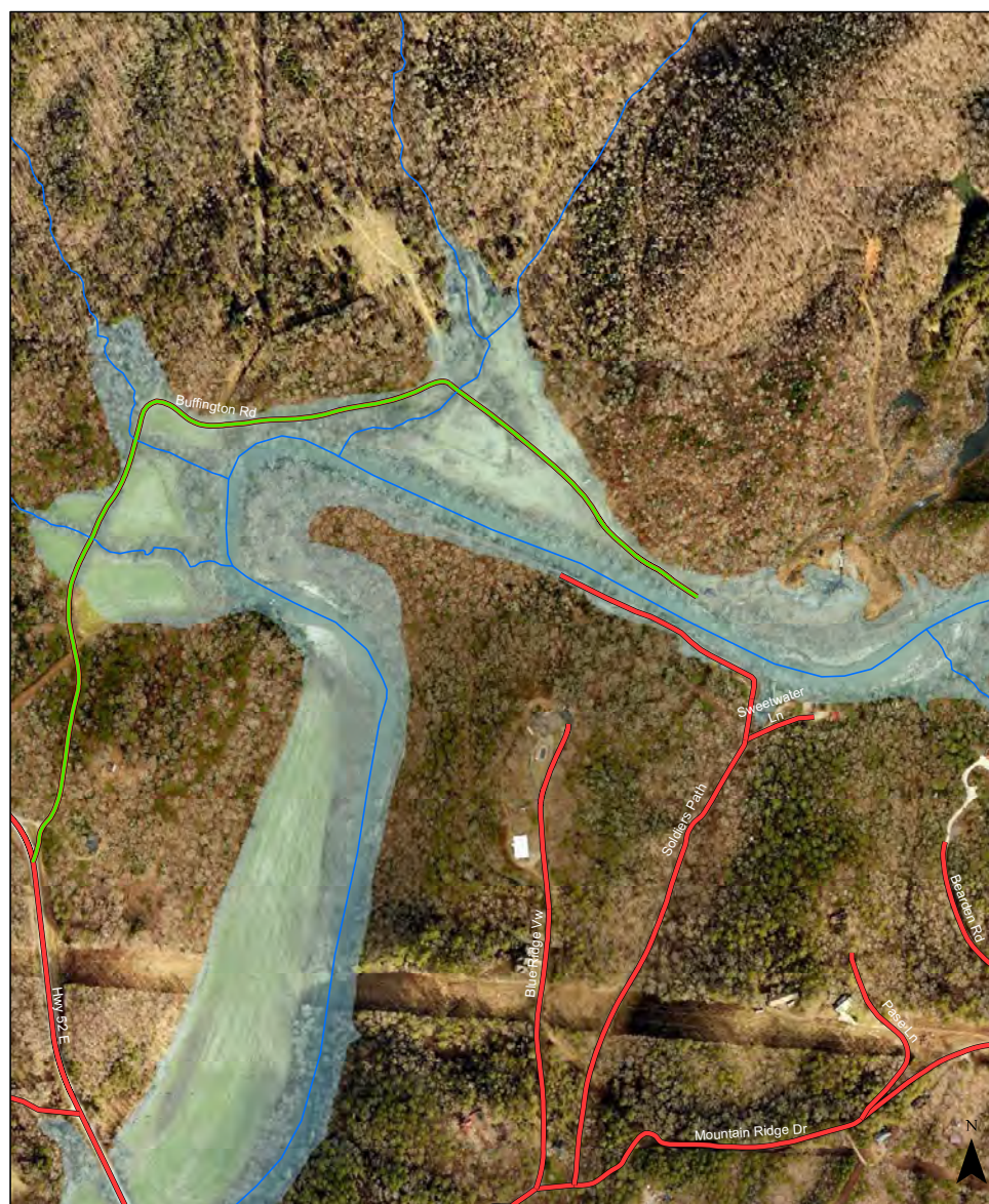
Flooding Concerns 12" over Buffington Rd.
